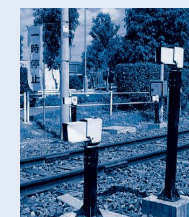
踏切障害物検知装置 Crossing Obstructing Detector
