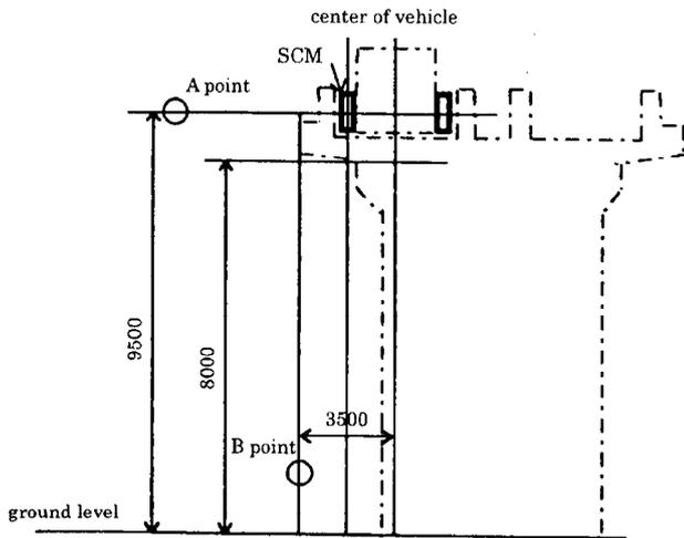
**Fig. 3 Cross section of standard viaduct (unit : mm)**
