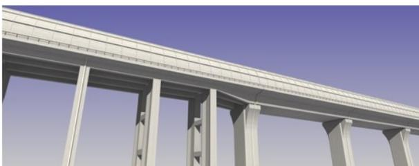
擦り付け部設置案(不連続性を桁部で処理)
